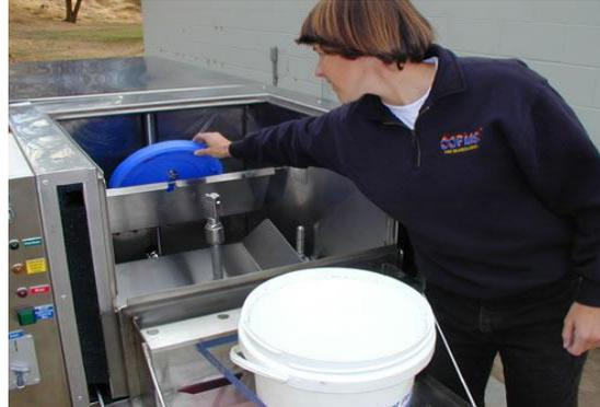
The wash hopper door is then closed and the cleaning cycle is begun with the push of a button.
