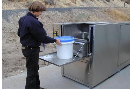
The user then removes the container lid, placing it in a different location in the machine for rinsing and sanitizing.
