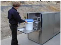
The user simply places the pail into the **SCAT MACHINE**; the pail is automatically emptied; and in less than two minutes the container is washed out, sanitized and ready for use again. The waste is properly disposed through sewage treatment methods.
